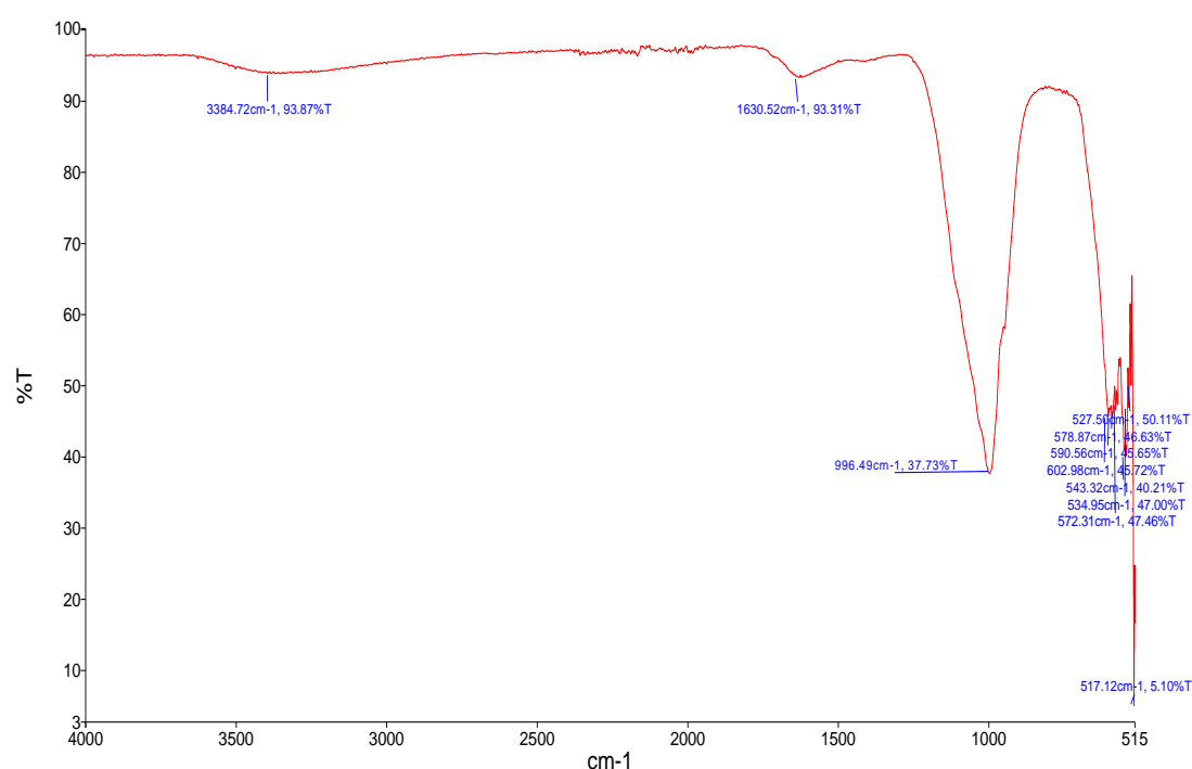
Fig. 10 FTIR spectra of MnO-NPs showing peaks at different wavelengths.
