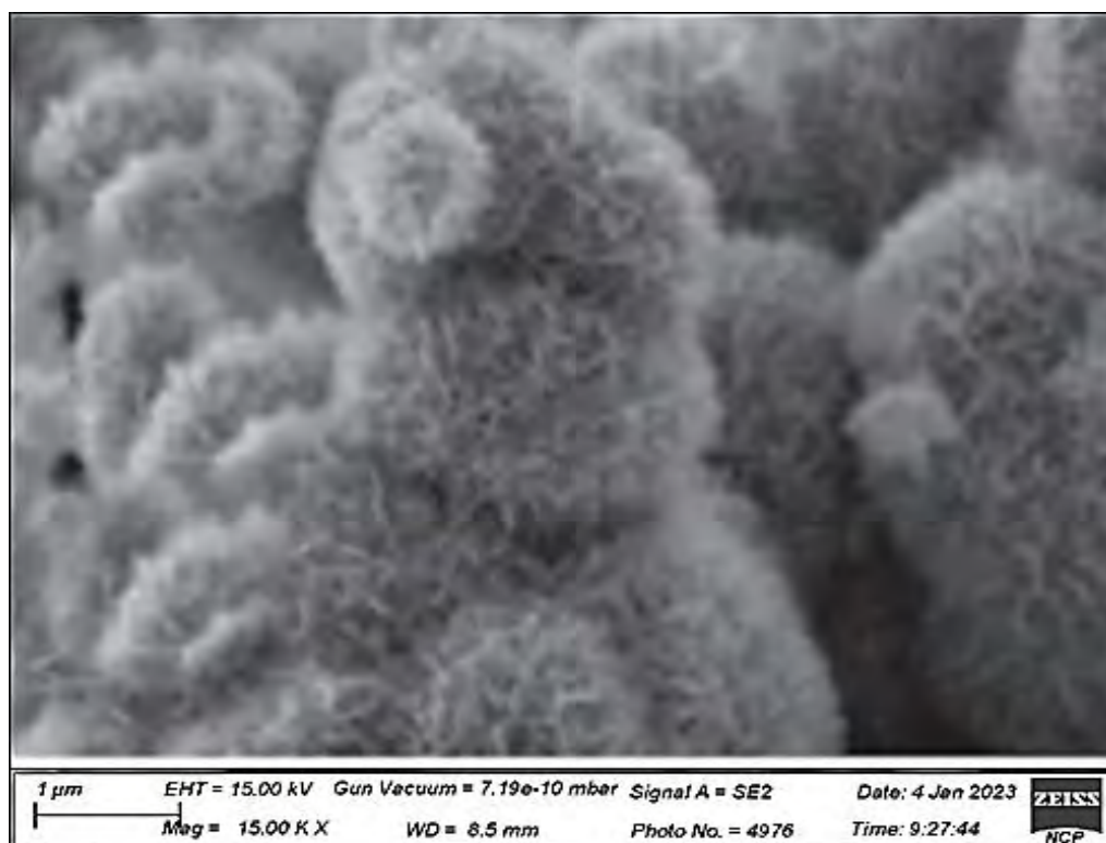
Fig. 12 Scanning electron microscopic photograph of MnO-NPs prepared in B. subtilis .
