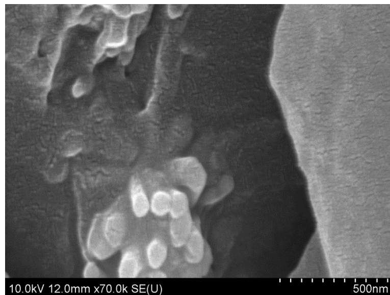
Figure 3.14 (b) SEM image of TTN 01-4, 2%ZnO NPs
