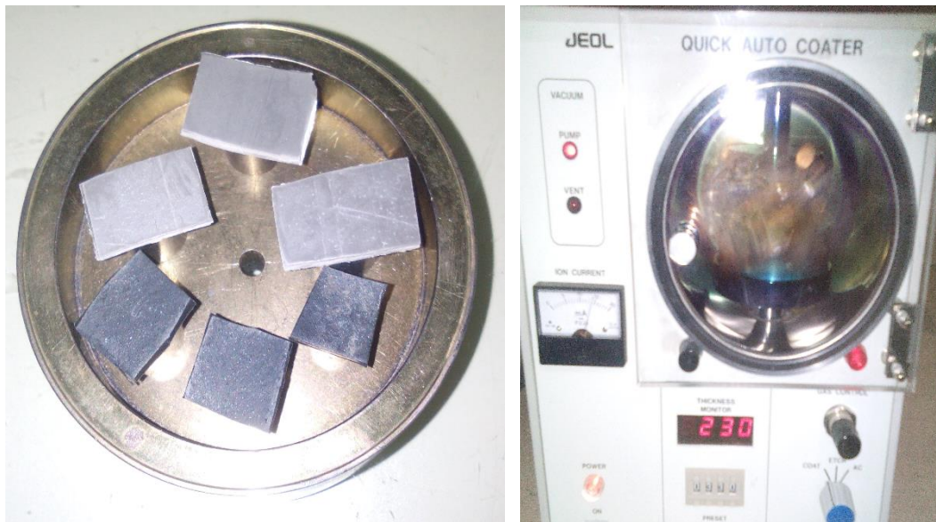
Figure 4.34. Biofilms on Polyvinyl chloride (PVC) and tire rubber (TR) (left; before scanning electron microscopy on stud, right; biofilm samples inside ion sputtering device for gold deposition on the surface of biofilms)
