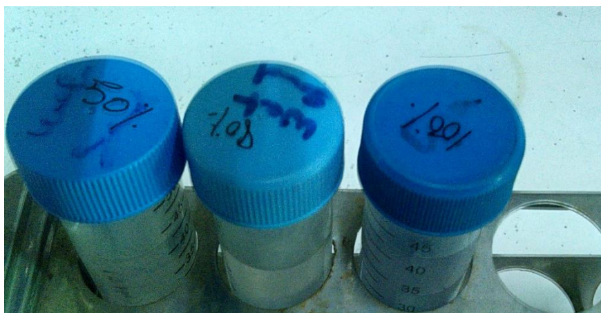
Figure 3.4. Series of different percentages of ethanol for dehydration of ten well glass slides (50%, 80%, 100%)
