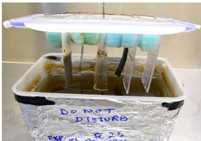
Figure 4.8 An aerobic batch biofilm reactor (ABBR) after biofilm development on different support materials with supplementation of Fe-2.5 mg/l.
