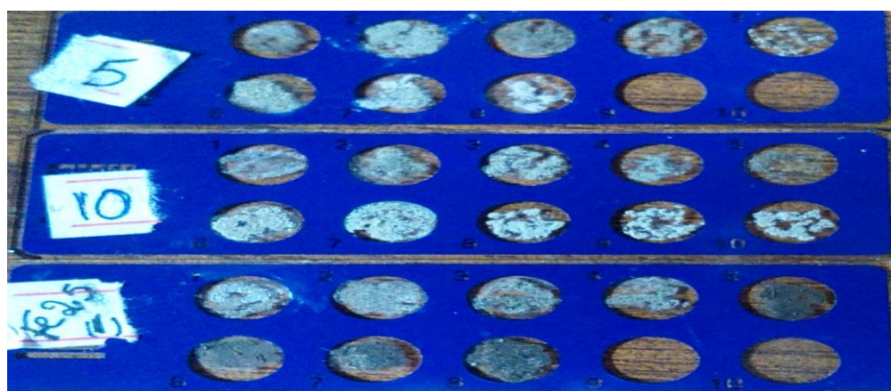
Figure 4.39. Teflon coated ten well glass slides after fixation of biofilms developed on different support materials under varying Fe(III) concentrations.
