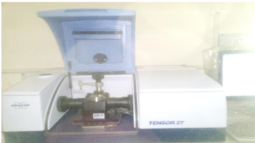
Figure 4.28. TENSOR 27 Fourier Transform Infra-red Spectroscope used for characterization of extracellular polymeric substances (EPS) of biofilms developed on different support materials under varying concentrations of Fe(III)
