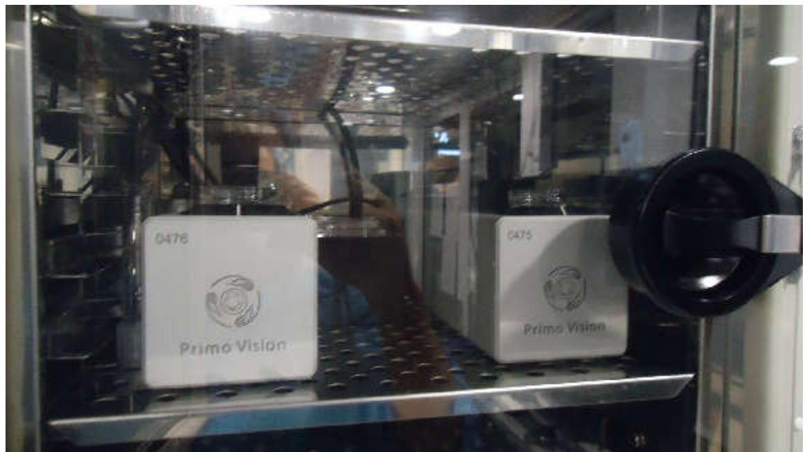
Figure 5.2. The Primo Vision group cultured dish placed on Time-Lapse microscope in an IVF incubator.
