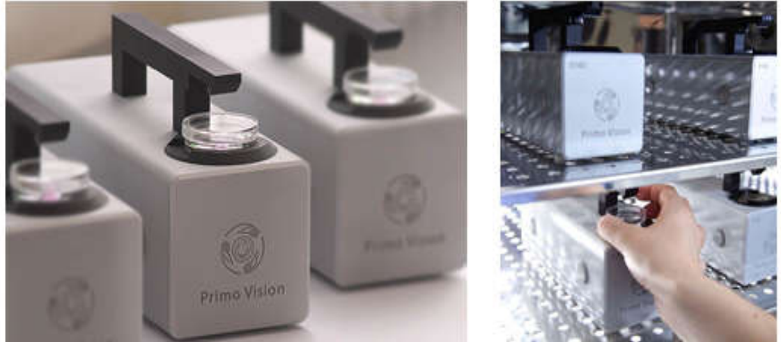
Figure 4.1. Using the Primo Vision group culture dish for time-lapse evaluation of embryos.
