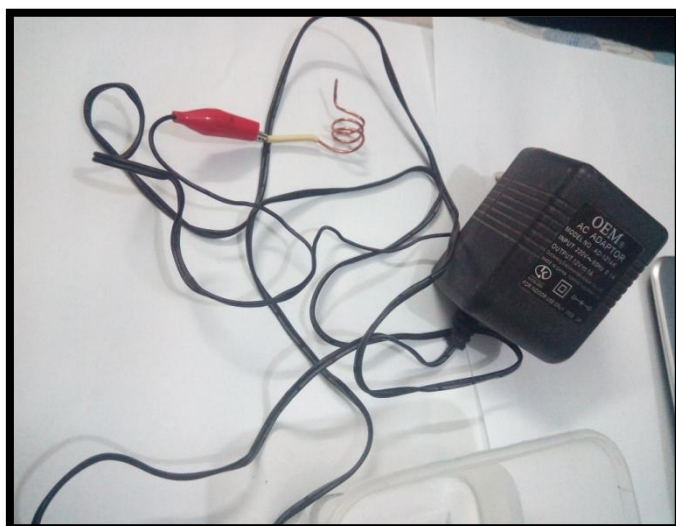
Fig 3.45: Transformer with Copper wire
