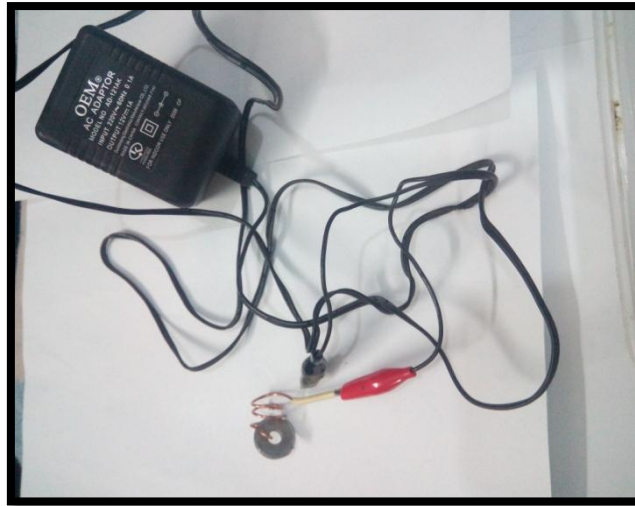
Fig 3.46: Transformer along with copper wire and steel washer
