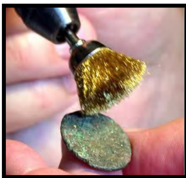
Fig 3.17: The Soft-bristle Brass Brush... the Correct Way!
