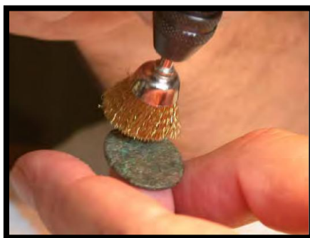
Fig 3.16: The Soft-bristle Brass Brush... the Wrong Way!
