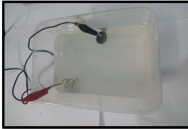
Fig 3.48: Transformer with ionized solution
