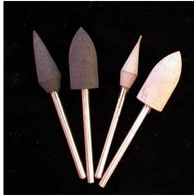
Fig 3.32: Diamond dusted rubber tools ‘Black Arrow (BA), Black Bullet (BB) and Gray Bullet (GB), Gray sharp Point (GSP)’
